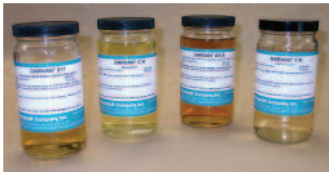
Deflocculants are added to slip to create chemically coated and charged particle surfaces. Photo courtesy of R.T. Vanderbilt, Co. Inc., Norwalk, Conn.
