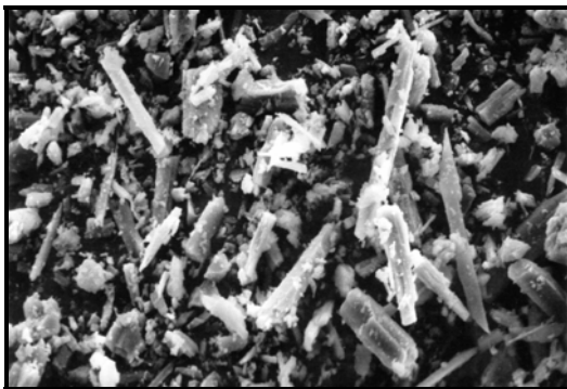
VANSIL Wollastonite: acicular, prismatic/nodular
