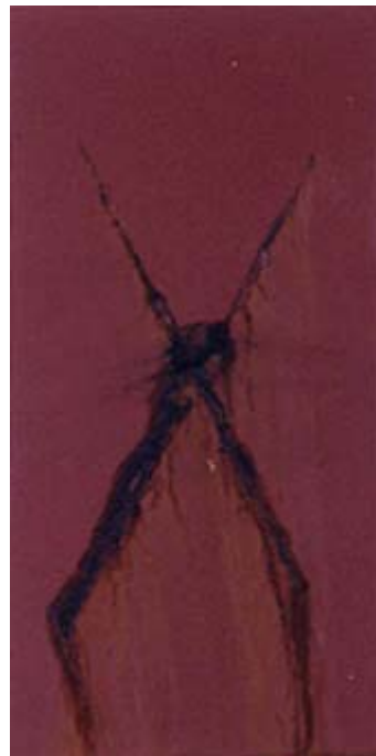
Formula 082101 B Fast Dry Shop Primer Competitive epoxy-silane treated 1250 mesh wollastonite 1008 hours
