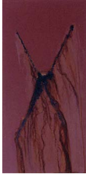
Formula 082101 A Fast Dry Shop Primer Competitive untreated 1250 mesh wollastonite 1008 hours
